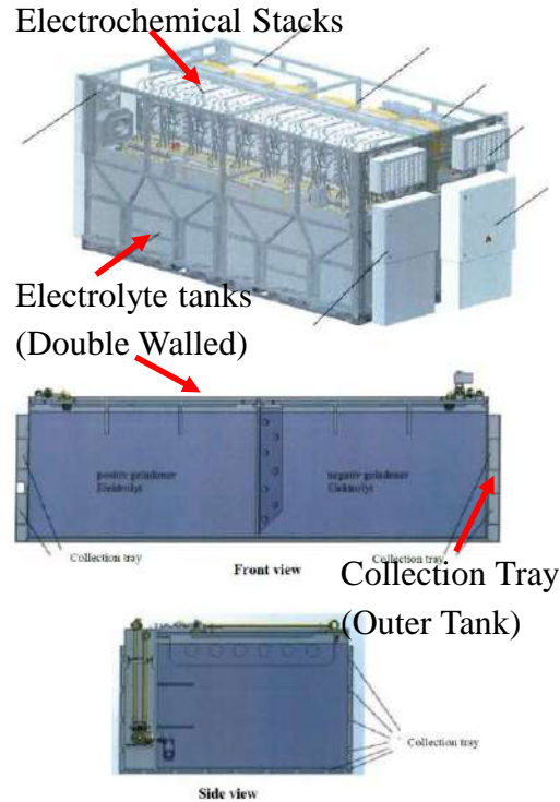
Double Walled Electrolyte Tank for Spillage Control
